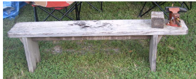
A low to the ground Bow Bench with a small vice.
