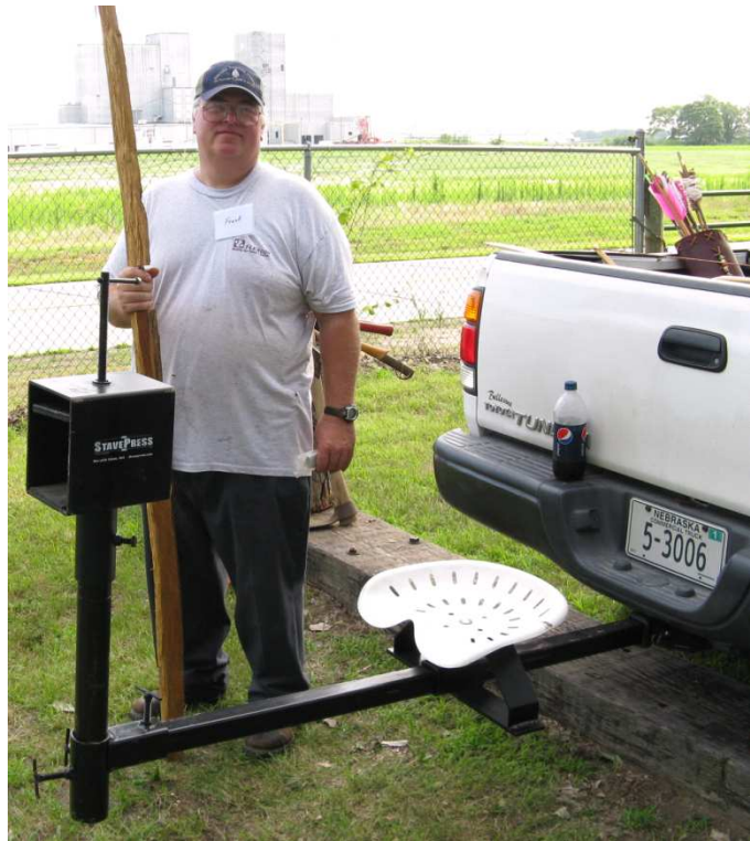
Frank Hicken won the "Most Unusual Bow Horse" award. He named his unique creation "The Bohemian Bow Horse". Note that it has no legs. The horizontal bar simply attaches to a pickup receiver. The Stave Press and tractor seat are both fully adjustable. Frank claims that his unique design is completely tested and that it is so flawlessly engineered that he can effortlessly work on an osage stave while his son Zack is driving down a rough gravel road at 50 miles per hour. We are still awaiting a photo to prove that claim.
