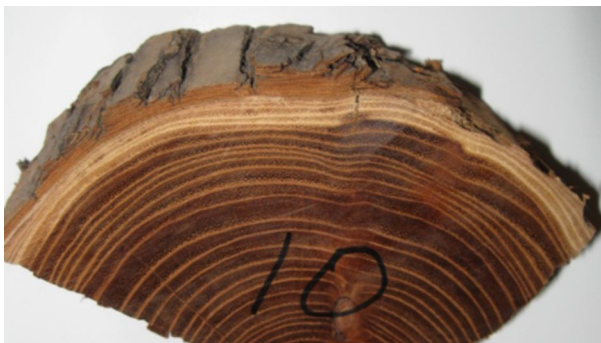
Bark covers the lightest area, the sap wood. The thin light colored rings are the Spring Growth. The wider darker colored rings are the Summer Growth. This stave has about 10 growth rings per inch.
