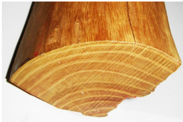
Bark and sap wood are removed from this osage stave and it has been taken down to a single growth ring. The thin lighter colored rings are Spring Growth. The wider darker rings are Summer Growth. This stave has about 4 growth rings per inch.
