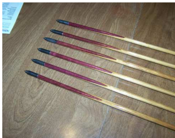
Purpleheart footings were added to lengthen the shafts to 32-1/2".
