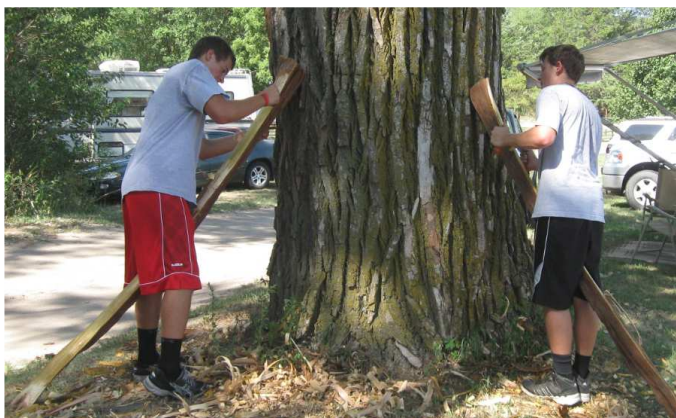
Two young bowyers, Dalton Hand and Brandon Klein are employing the most efficient method to remove bark and sapwood from osage staves. Experienced self-bowyers know that standing the stave upright and letting your body weight and gravity pull the draw knife through the wood is easier than putting the stave in a bow horse and using just your back, and arm muscles as the only force to pull the draw knife through the wood.
