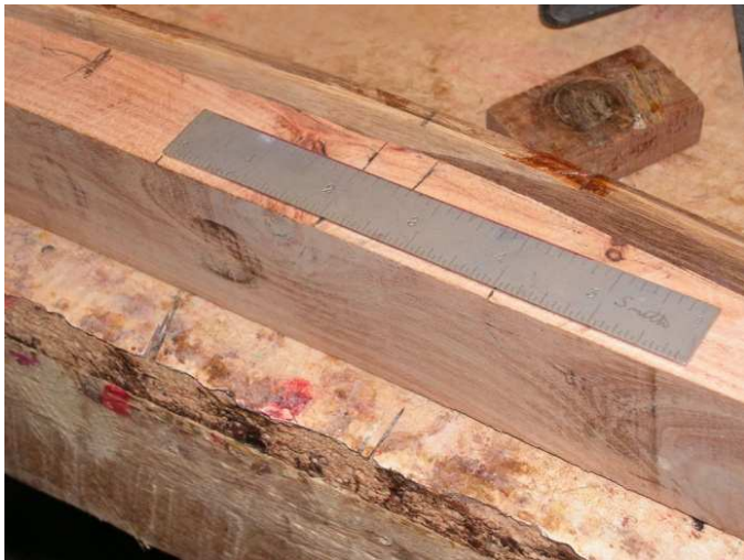
Laying out the 4-inch handle.
