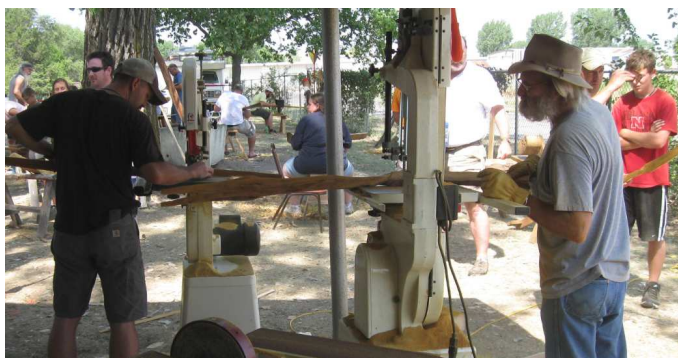
At left, Brandon Abbott cuts out a stave on the club's new Grizzly band saw, which was a real workhorse over the weekend. At right, Todd Nielsen cuts out a stave on Ken Oberschulte's JET band saw.
