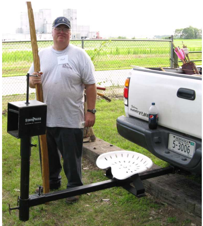
Frank Hicken won the “Most Unusual Bow Horse” award for the second year in a row. Frank’s unique creation is known as “The Bohemian Bow Horse”. Note that it has no legs. The horizontal bar simply attaches to a pickup receiver. The Stave Press and tractor seat are both fully adjustable. Frank claims that his unique design is completely tested and that it is so flawlessly engineered that he can effortlessly work on an osage stave while his son Zack is driving down a rough gravel road at 50 miles per hour.
