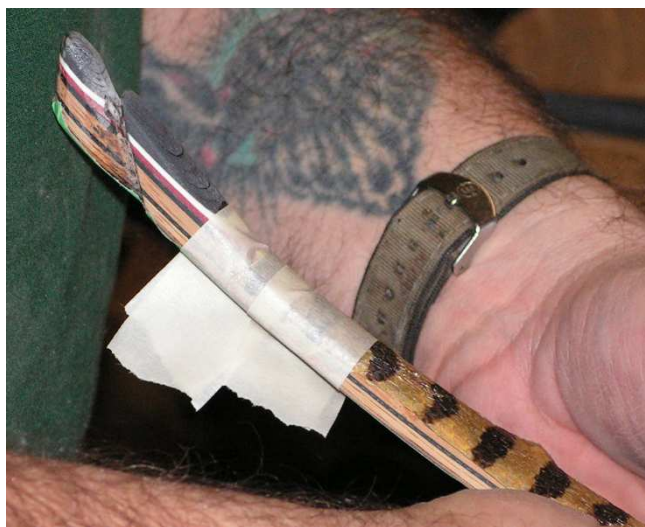
The first tape downs, one inch masking tape secures the snake skin to the limb at the nock end.
