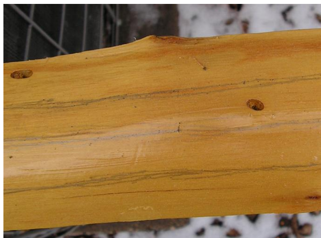
Wood wasp holes in back of osage stave.
