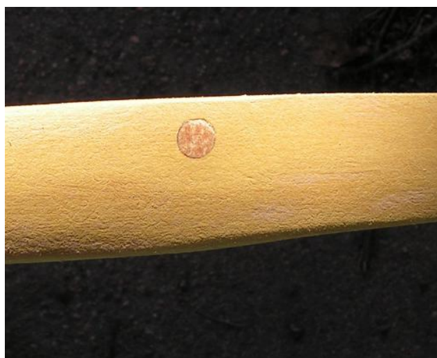
Dowel plug cut off and sanded down to be flush with surface of the back of the bow.
