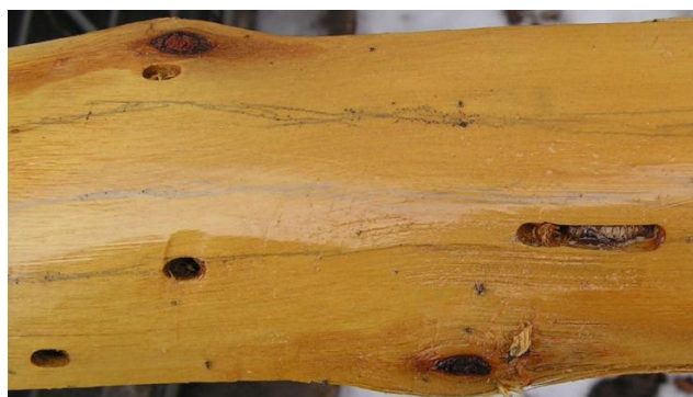
A wood wasp still in elongated hole in back of stave.
