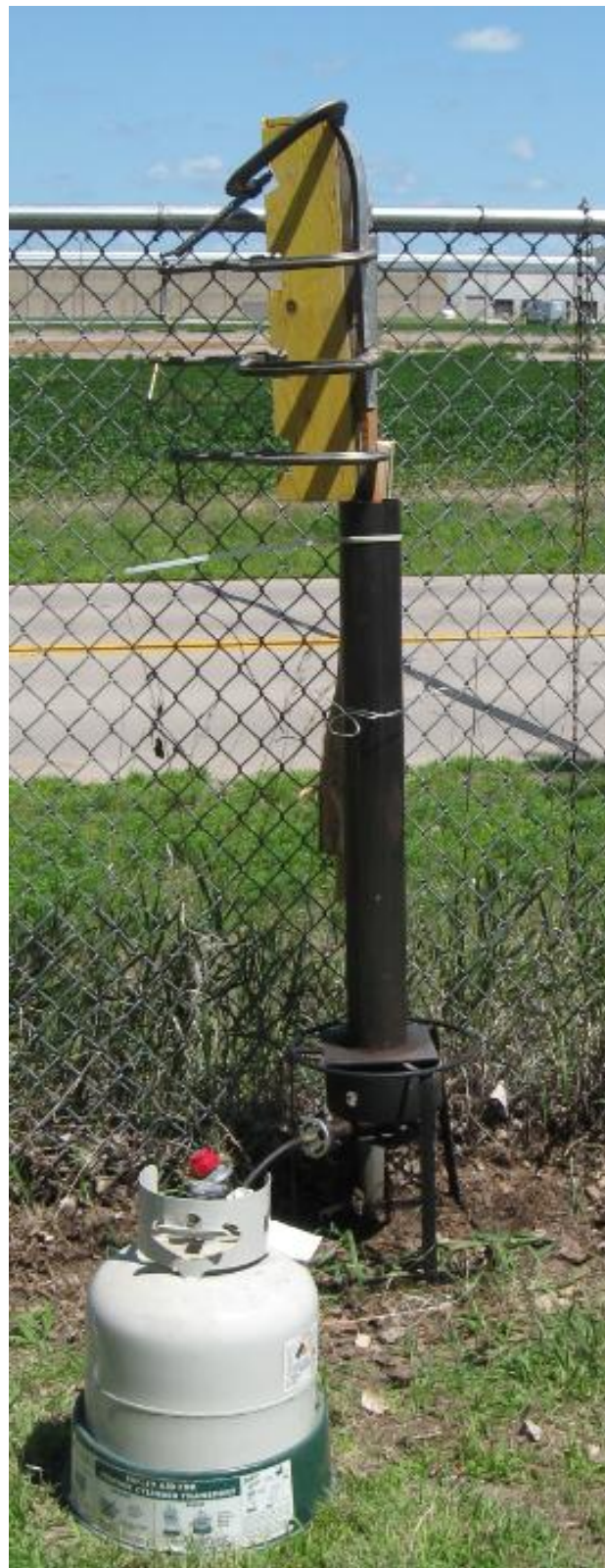
This homemade boiling tube is being heated on a propane turkey cooker. Top limb is clamped to a recurving form as bottom limb is in the boiling tube. Note boiling tube is secured to the chain link fence so it cannot tip over off of the turkey cooker.
