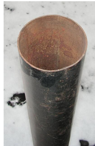
Boiling Tube, 4" diameter thin walled steel tube 48" long.
