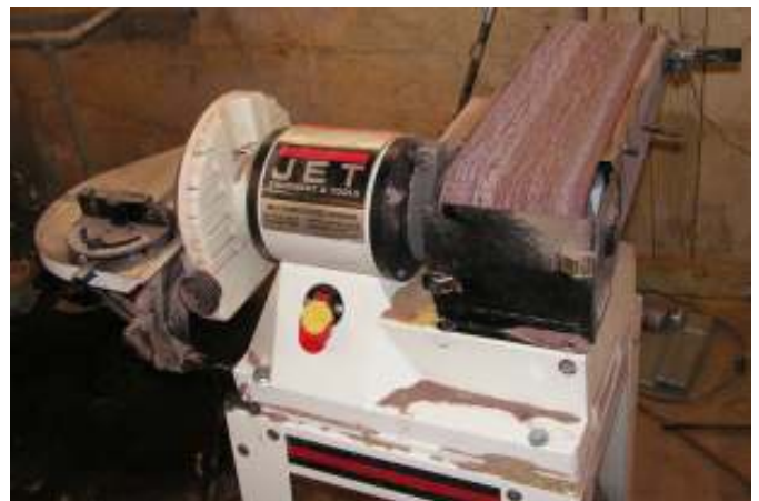
A free standing sander combo with a 6"x48" belt and 10" disc.
