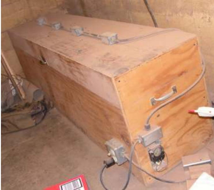
This bow oven is a large item. It is 8' long x 1' wide x 2' deep. Bow ovens are usually placed in an out of the way corner or nook of the shop.
