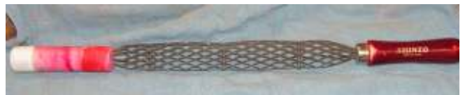
Above the standard 2-sided Shinto rasp has one handle, below an aftermarket second handle provides additional control and significant leverage to remove material.
