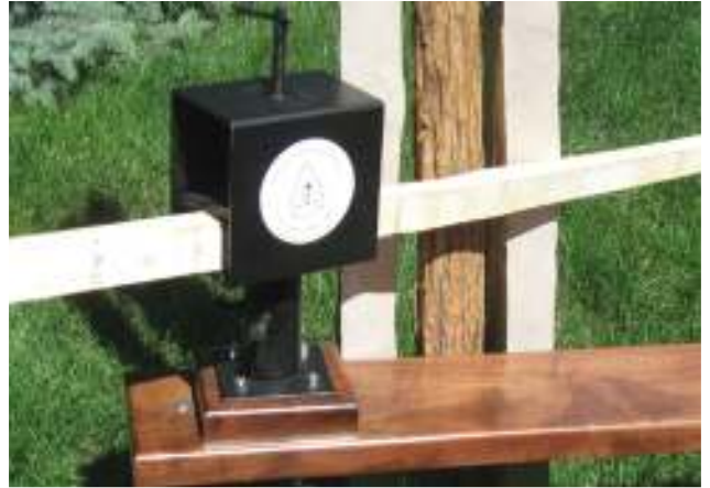
The heavy 5-1/2" x 5-1/2" plate steel base of a Stave Press can be mounted anywhere with clamps or bolts.
