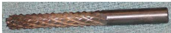
Above is the versatile Dremel tool. Below is a tile cutting bit for cutting string notches and shaping bow tips.
