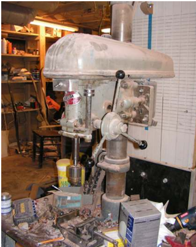
A drill press is used for drilling holes for takedown bows.
