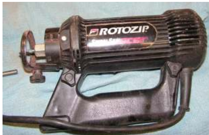
The Roto-Zip with a tile cutter bit is a quick and even way to cut out a shelf in a fiberglass laminated bow.
